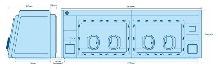
**Important note:** If the **Refrigeration System** is fitted, please allow a clearance of 770mm behind the workstation. If the **Heat Removal System** is fitted, please allow a clearance of 600mm behind the workstation. Some of this clearance is necessary for air circulation.
